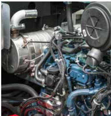
Tier 4/Stage V ready engine with built-in diesel particle filter and catalyst
